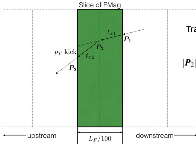
$$\text{Track slope in XZ plane: } t_{x2} = t_{x1} + s \cdot \frac{\text{kick}}{L_{\text{FMag}}} \cdot \frac{L_{\text{FMag}}}{N_s} \cdot \frac{1}{\sqrt{P_{1x}^2 + P_{1z}^2}},$$
